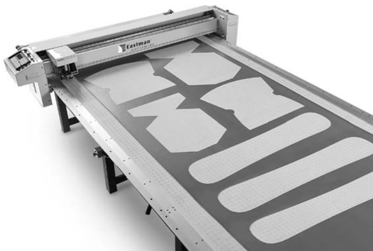
Fig. 17 View of a small automatic prepreg cutting machine. This shows how the plies have been positioned to minimize wastage. (Photograph by courtesy of the Eastman Machine Co., Rochester, NY, Model M9000)
