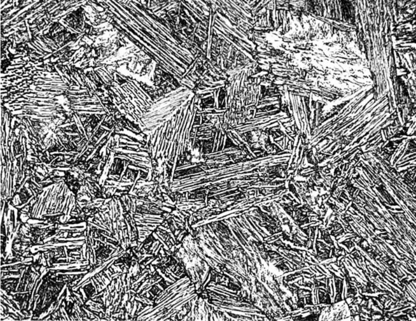
Fig. 8 Photomicrograph of a low-alloy steel showing a bainitic microstructure. 500X. 4% picral + 2% nital etch.
