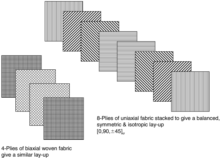
Fig. 14 Uniaxial reinforcement, such as prepreg, must normally be laid up in a balanced, and symmetric sequence. This requires eight plies to give an isotropic laminate. If balanced woven reinforcement is used a similar effect may be realized with just four plies.
